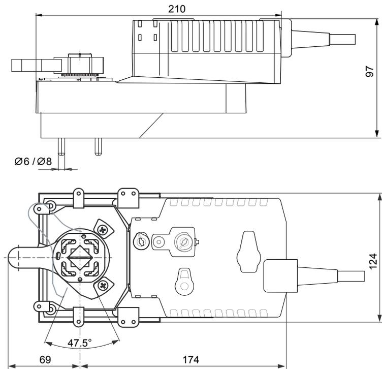
**Modulating rotary actuator for rotary valves**
