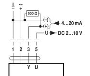
Control with 4...20 mA via external resistor
